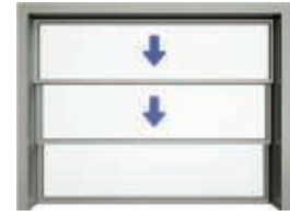
Window with two sliding sections opening downwards
